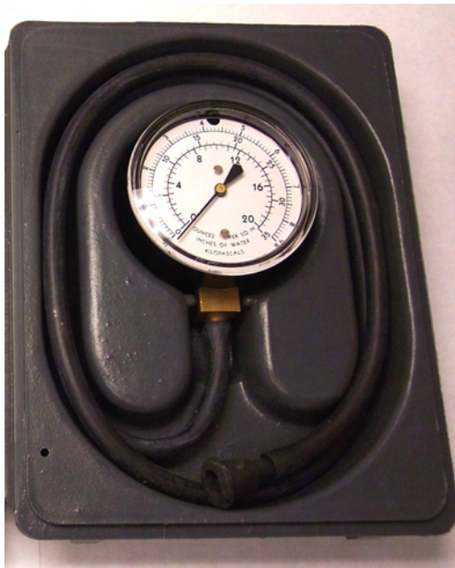
Low Pressure Manometer
