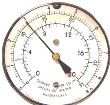
Regulated Propane inlet pressure should be: 12” of water column
